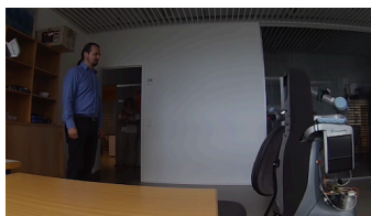
The robot starts to drive, says "please put your finger into the sensor" , and extends its arm with the sensor
